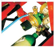
An adjustable pressure reducer provides the service pressure of 4.5 to 6 bars required for the actuators.
