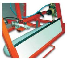
Numerous quick release, adjustable devices allow the starting gate to be quickly adjusted to suit any type and size of bicycle.
