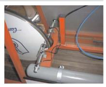
Two pneumatic actuators grip the cycle's rear wheel with a pressure of 4.5 to 6 bars. The pneumatic energy is provided by a bottle of gaseous nitrogen at a pressure of 200 bars.
